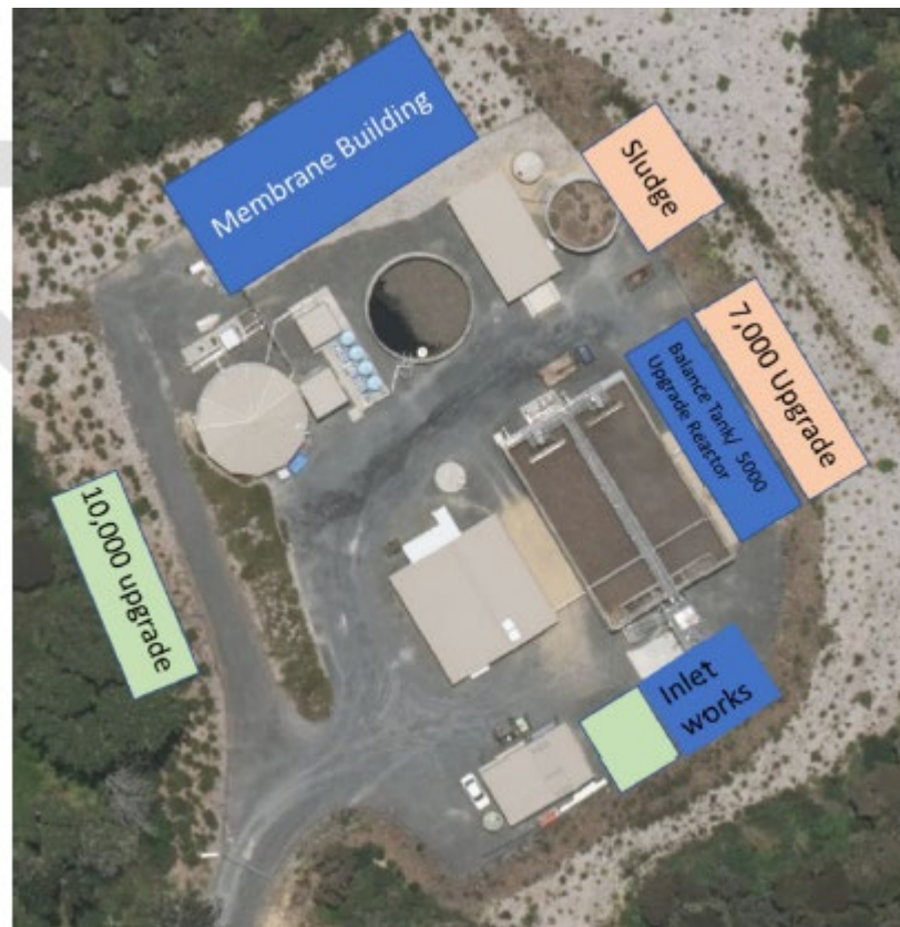
Figure 5 : Tank Concept Layout of CWWTP Upgrades to 10,000 connections
